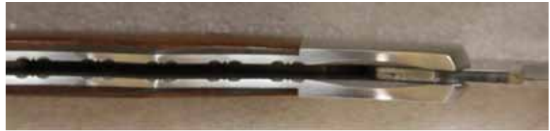
Close-up of 531 Sawby type frame with convex bevel cutout used on first mid-body lockback models.
